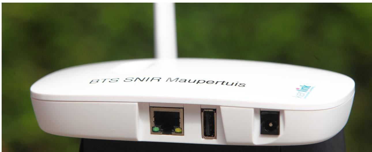
Figure 4: Gateway LoRaWAN Kerlink iFemtoCell
