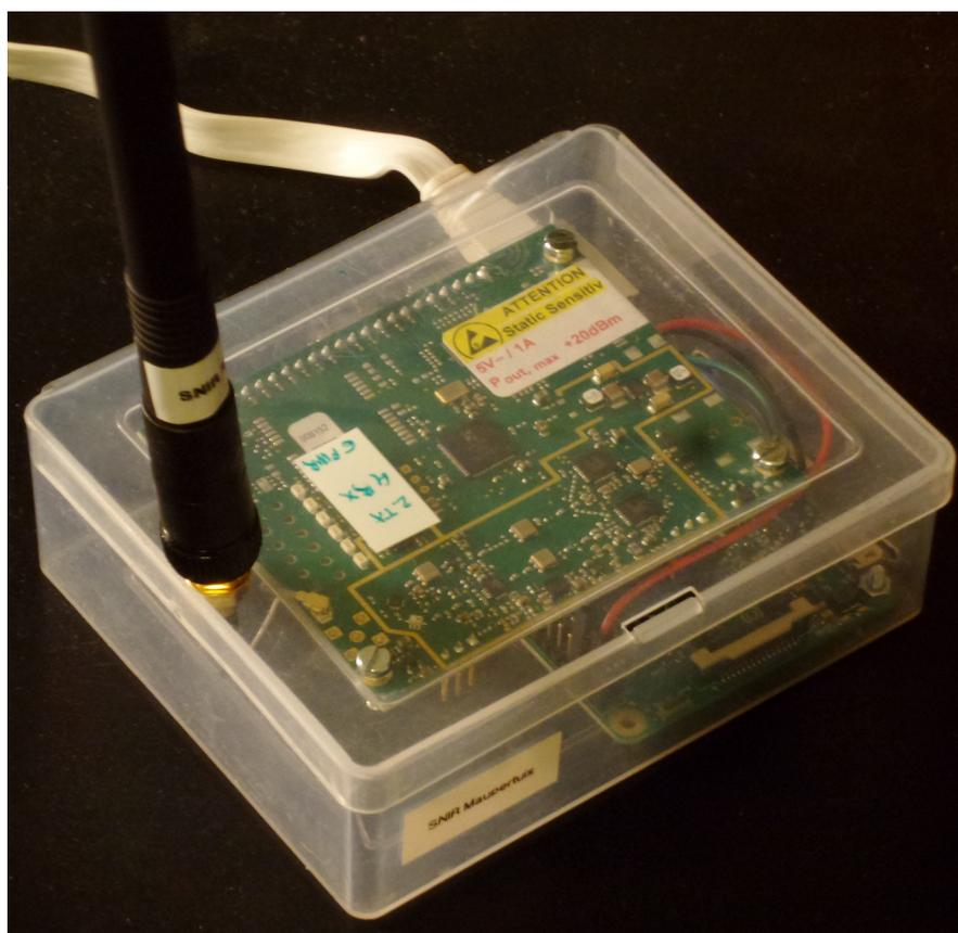
Figure 5: Gateway LoRaWAN DIY IMST + Raspberry
